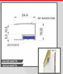
Frame made of aluminum profile with various types of coating, intended for placement of medium size images.
